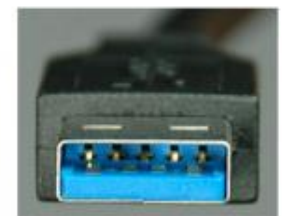
USB 3.0 A plug pinout
