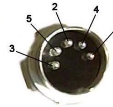
AT keyboard connector (DIN5)
