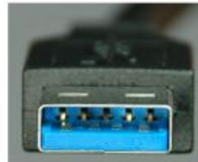
USB 3.0 A plug pinout
