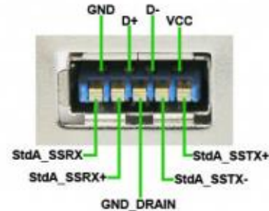
SuperSpeed standard A plug pinout
