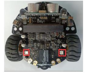
**Principle**: LED light (red, green, blue) are packaged in the LED module. We can mix different colors(256\*256\*256) by controlling the brightness of the three LEDs.
