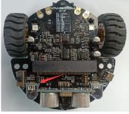
In the picture shown below, the voice sensor module with red wire frame.
