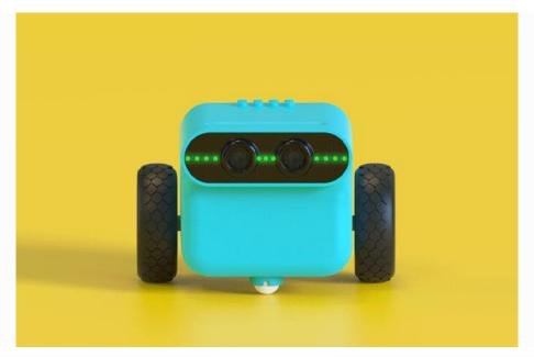
• While in its line-tracking & obstacles-avoidance mode, the headlights turn to red and it stops moving if an obstacle was detected.
